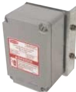
*Chore-Time's Auger Timer can be used to prevent the auger system from running longer than a pre-set time between 3 and 100 minutes. The timer prevents the system from running empty for long periods of time. For added protection, system requires a manual re-set after activation.*
