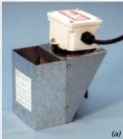
*The mechanical Hopper Level Control (a) is used to maintain the feed level in the hoppers for continuous feed supply.*
