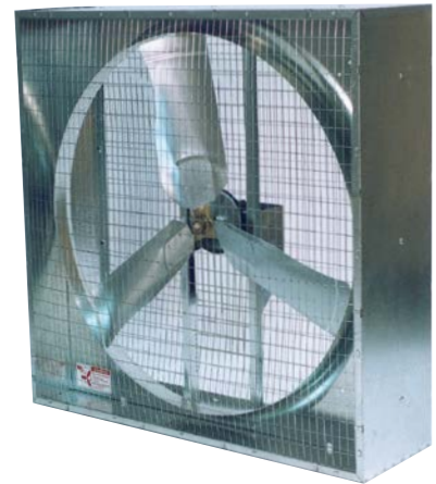
Chore-Time's 36-inch Direct-Drive Box Fans deliver 10,980 CFM and 16.4 CFM/Watt at 0.00 static pressure.
