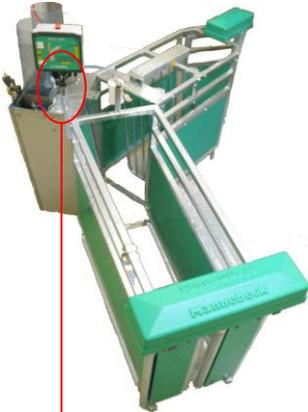
Connection Zx through a Y-cable for feeder control
