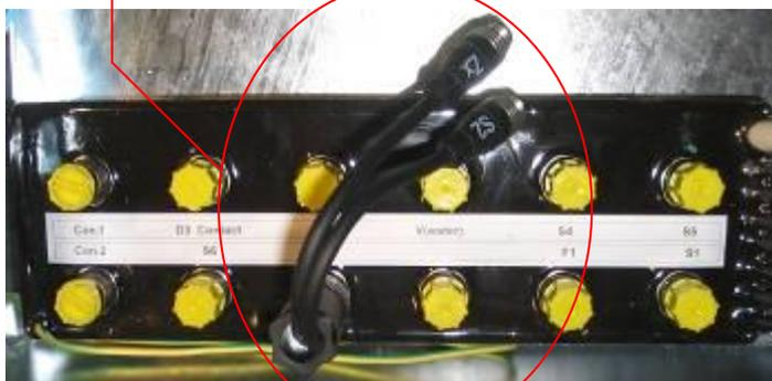
Release the cable for the entrance sensor from the S2/Z1 socket of the INTEC MAC. Then plug the Y-cable onto the S2/Z1 socket and connect as follows:
