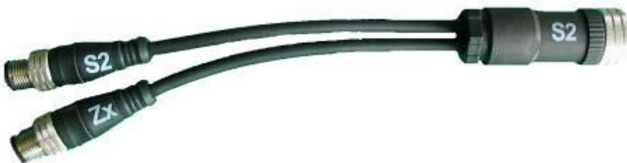
To connect a feeder control to the INTEC MAC, a Y-cable is added at the connection of the entrance sensor S2/Z1 by disconnecting the entrance sensor cable from the INTEC MAC and connecting it to plug S2 of the Y-cable. The feeder control is connected by means of the plug ZxZx.
